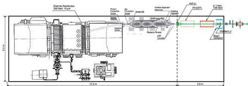
Fig. 1. An example of a compact muon source using a 300-MeV electron microtron.
