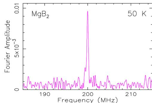
Fig. 1: Fast Fourier Transform of  $\mu$ SR spectrum over a time region from 1.5  $\mu$ s to 6  $\mu$ s (where the RF noise is negligible) obtained from a time spectrum.
