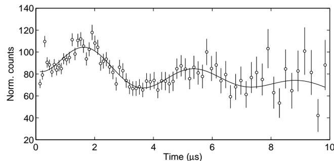
Fig. 1: MuSR signal at 20 G TF measured with a *single* scintillating fiber.
