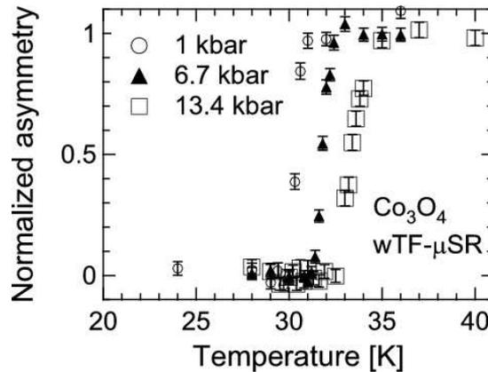
Fig. 1:  $T$  dependences of  $A_{\text{TF}}$  for  $\text{Co}_3\text{O}_4$  under three different pressures.
